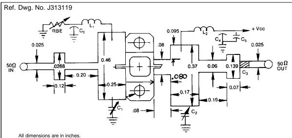
Substrate material: .025 thick Al<sub>2</sub>O<sub>3</sub>
